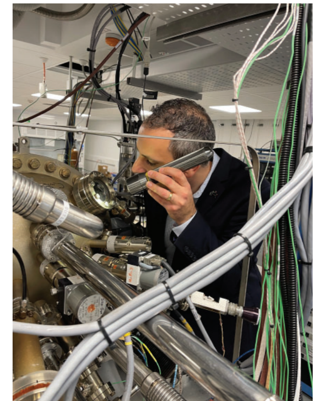
ABOVE DR ENRICO PALERMO TAKES A GOOD LOOK AT THE MOLECULAR BEAM EPITAXY MACHINE IN THE AVIONICS LAB.
