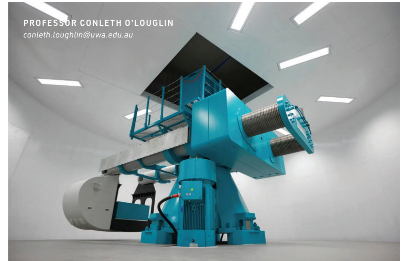
ABOVE 10M CENTRIFUGE HOUSED AT UWA'S CENTRE FOR OFFSHORE FOUNDATIONS SYSTEM BELOW LEFT PROFESSOR CONLETH O'LOUGHLIN EXPLAINING TESTING SYSTEMS IN THE NGCF BELOW RIGHT ADAM STUBBS DEMONSTRATING THE 3.6M CENTRIFUGE.
