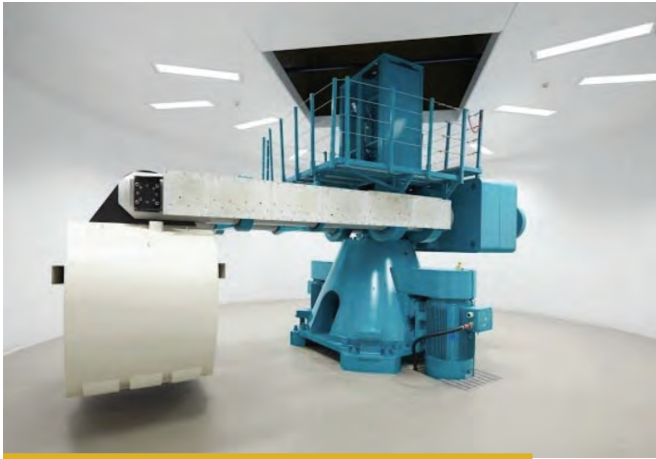
ABOVE 10m Centrifuge housed at UWA's Centre for Offshore Foundations System
