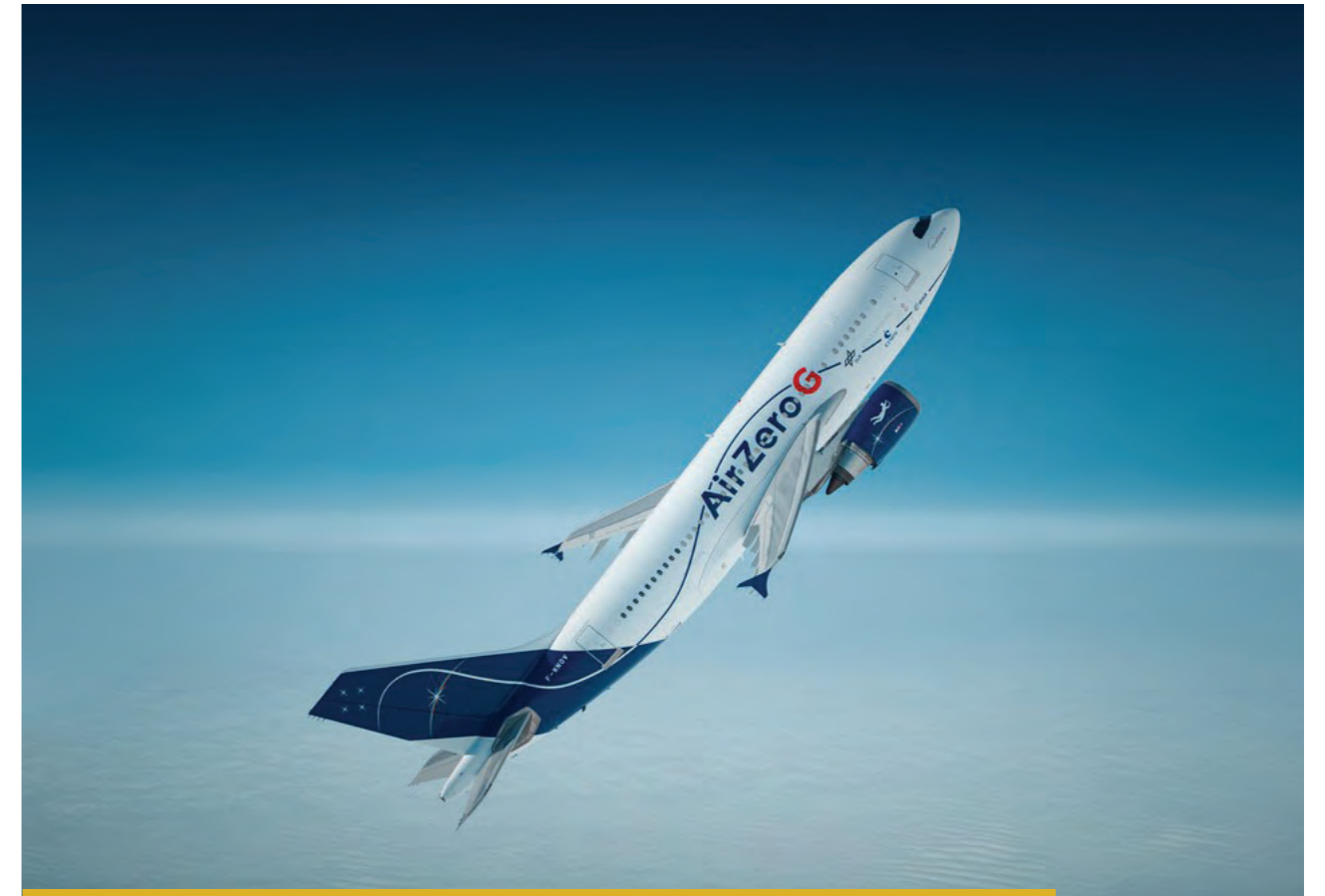
ABOVE Novespace's Zero-G A310 Airbus, modified to perform science experiments in microgravity.
