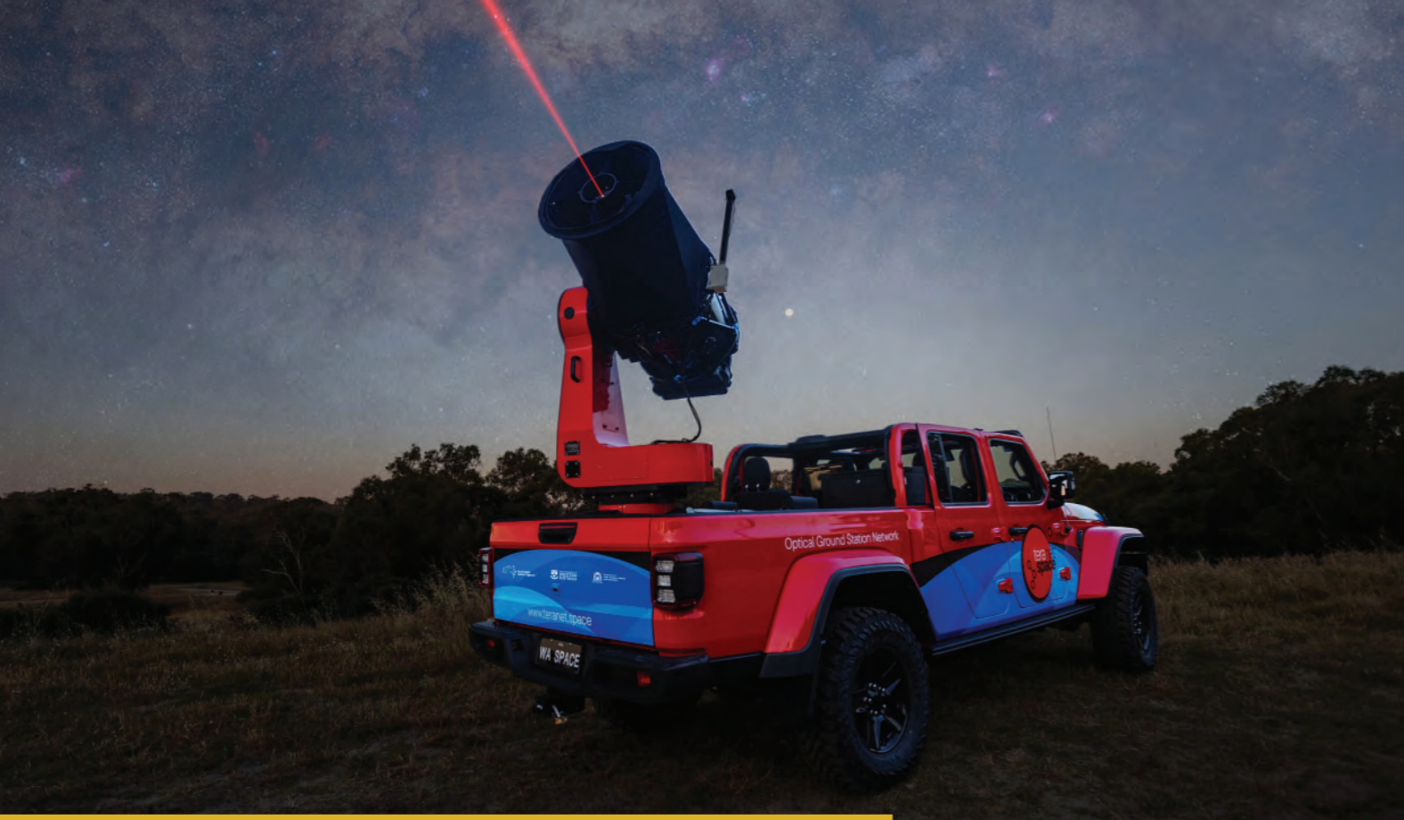
ABOVE TeraNet-3 running a tracking and acquisition demo on the ISS (Image – the Bold Park astro image of the Jeep taken by Michael Goh, edited by Aliesha Aden)
